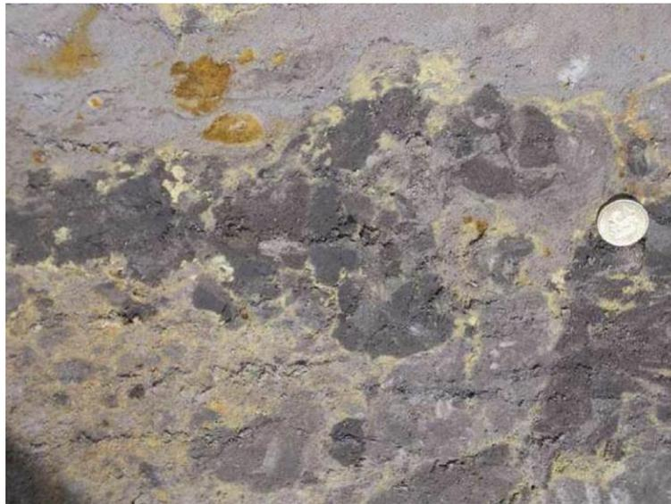
Figure 4. Shallow excavation into dredge spoil that has been deposited at Murray Waters Boulevard in South Yunderup showing mottles of jarosite (yellow colour), ferruginous mottles and remnant unoxidised sulfidic material (dark grey)(Photo: Leigh Sullivan).
